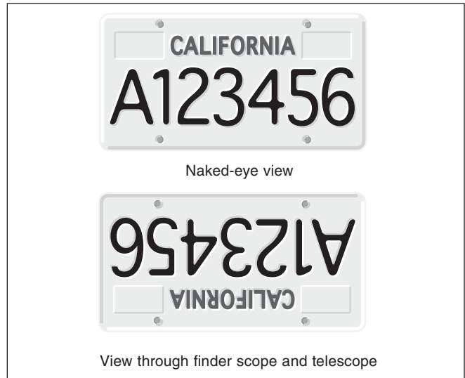
Figure 5. The view through a standard finder scope and reflector telescope is upside down. This is true for the SpaceProbe 130ST and its finder scope as well.
