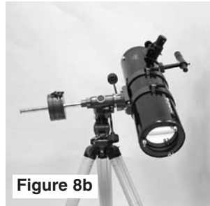
Figure 8a,b,c,d. This illustration shows the telescope pointed in the four cardinal directions: (a) North, (b) South, (c) East, (d) West. Note that the tripod and mount have not been moved; only the telescope tube has move on the R.A. and Dec. axis.
