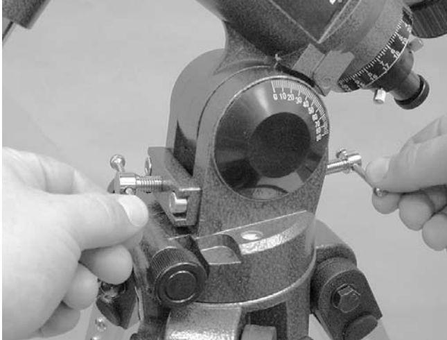
Figure 2. To adjust the latitude angle of the equatorial mount, loosen one of the two latitude adjustment T-bolts, then tighten the other.
