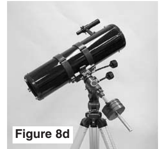
Figure 8a,b,c,d. This illustration shows the telescope pointed in the four cardinal directions: (a) North, (b) South, (c) East, (d) West. Note that the tripod and mount have not been moved; only the telescope tube has move on the R.A. and Dec. axis.
