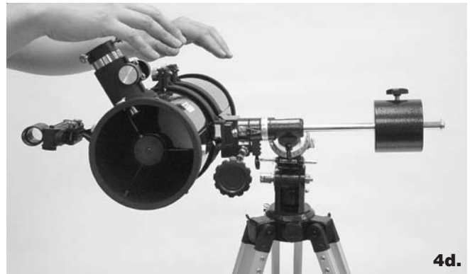
Figure 4. Proper usage of the equatorial mount requires the telescope tube to be balanced on both the R.A. and Dec. axes. (a) With the R.A. lock knob released, slide the counterweight along the counterweight shaft until it just counterbalances the tube. (b) When you let go with both hands, the tube should not drift up or down. (c) With the Dec. lock knob released, loosen the tube ring lock clamps a few turns and slide the telescope forward or back in the tube rings. (d) When the tube is balanced about the Dec. axis, it will not move when you let go.
