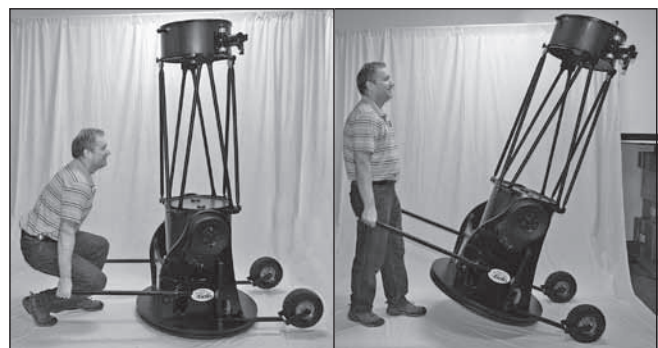
Figure 6. a) With the tube locked in the vertical position, lift the handles while keeping your knees bent and back straight, b) stand up and you're ready to roll!
