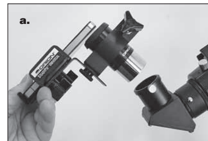
Figure 7. Inserting the eyepiece with adapter and phone attached into the star diagonal. Before doing this be sure that the diagonal is tightly secured in the telescope focuser!
