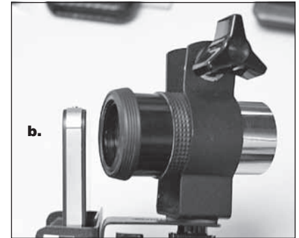
Figure 5. The eyepiece lens should be flat relative to the smartphone ( a ), not skewed at an angle ( b ).
