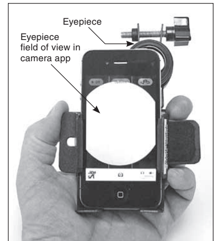
Figure 6. Position the telescope eyepiece so that its field of view appears roughly centered on the phone's screen.
