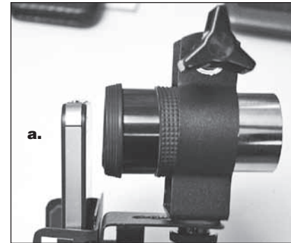
Figure 5. The eyepiece lens should be flat relative to the smartphone ( a ), not skewed at an angle ( b ).
