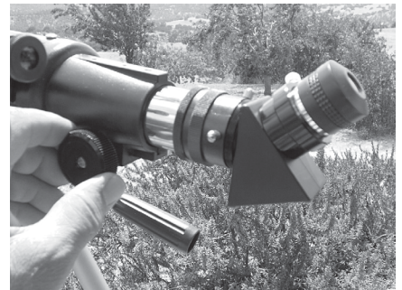
Step 8: Point the telescope towards a distant object; while looking through the eyepiece, turn the focus knob to adjust focus.
