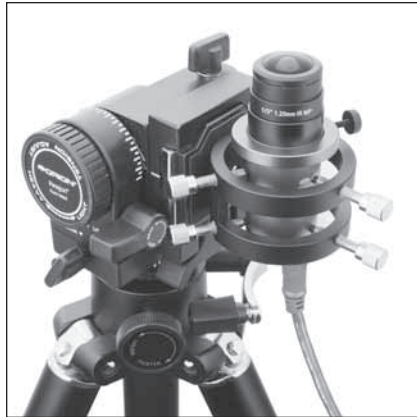
Figure 2. The SSAIO, Fish Eye lens and adjustable rings attached to a standard tripod.
