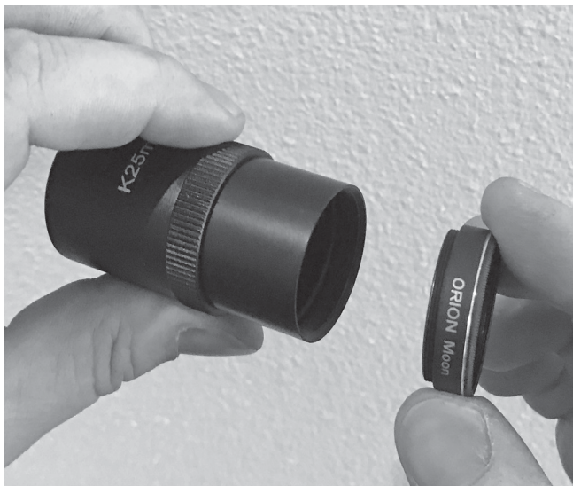
Figure 26. The Kellner eyepieces have barrels threaded to accept optional Orion 1.25” filters. A Moon filter is useful for cutting glare and revealing more detail on the lunar surface.
