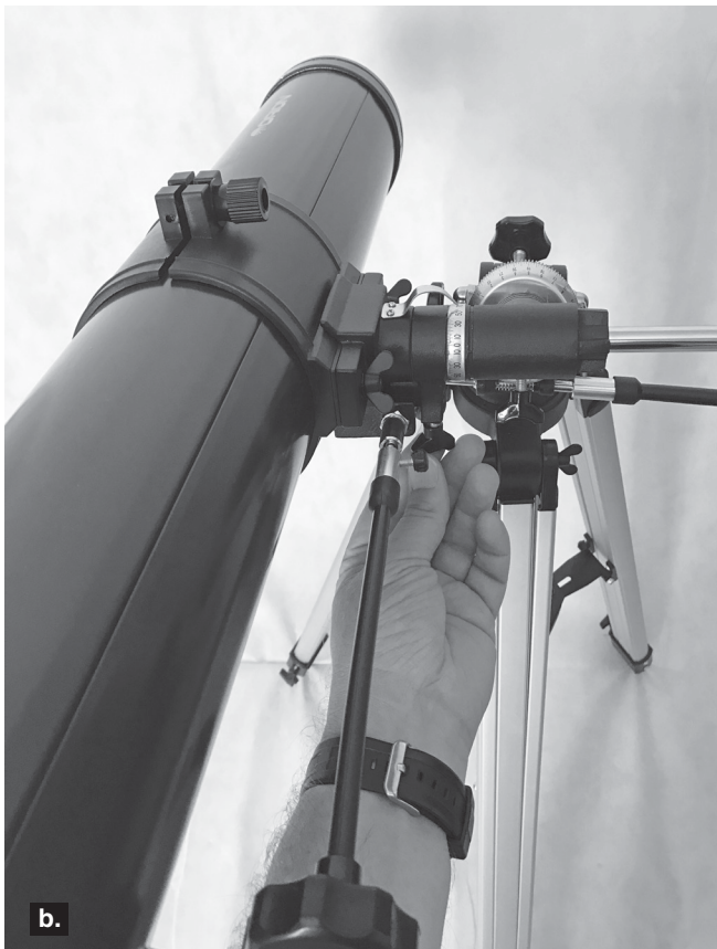
Figure 20. Balancing the telescope about the a) R.A. and b) Dec. axes.
