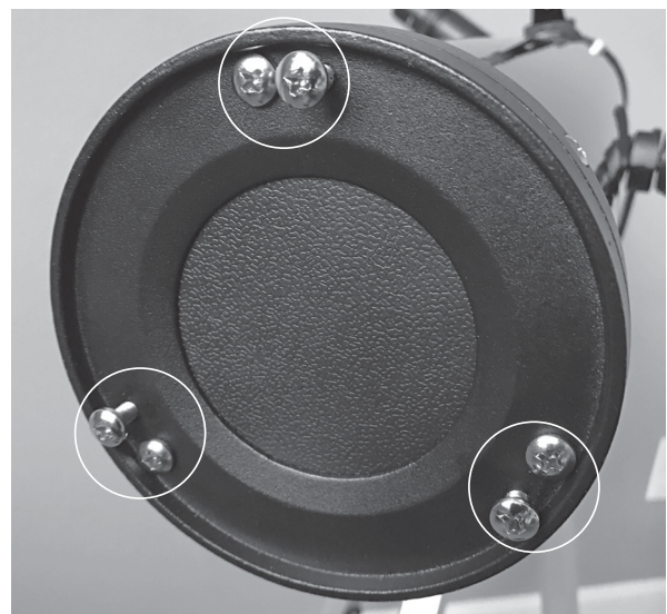
Figure 24. Align the primary mirror by adjusting the three pairs of “push/pull” screws on the back end of the optical tube.
