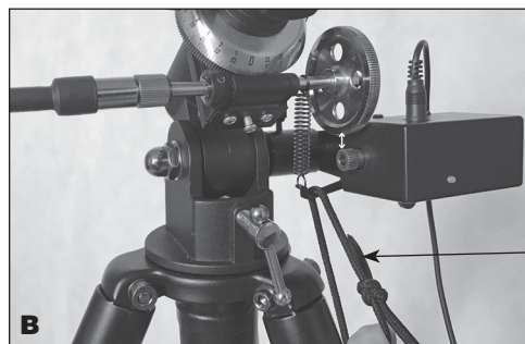
Figure 11 To move the right ascension axis with the slow-motion cable, disengage the motor drive by A ) pressing down on the motor housing using your hand, or B ) pulling down on the clutch cord.
